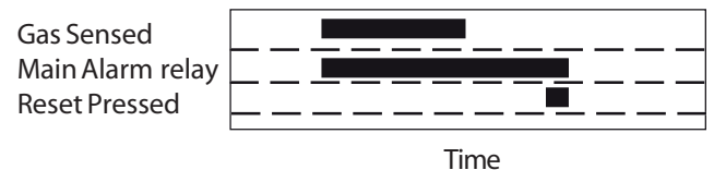
Main alarm switch in 'C' position
